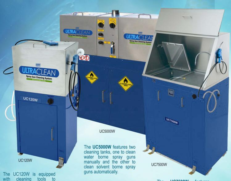
The UC120W is equipped with cleaning tools to manually clean spray guns with water.
